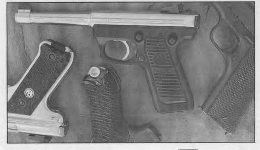
The magazine catch/release has been moved from the heel of the frame, where it is found on the standard Ruger .22 pistols in the European manner, to the left side of the frame directly in back of the trigger, where it is located in the M1911A1 series.
